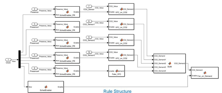
After the structure generation, the blocks are parameterized by varying optimization techniques and then transformed to a Simulink readable format so they can be used as a control strategy in the simulation. The simulation results are then used as feedback to the strategy generation process.
